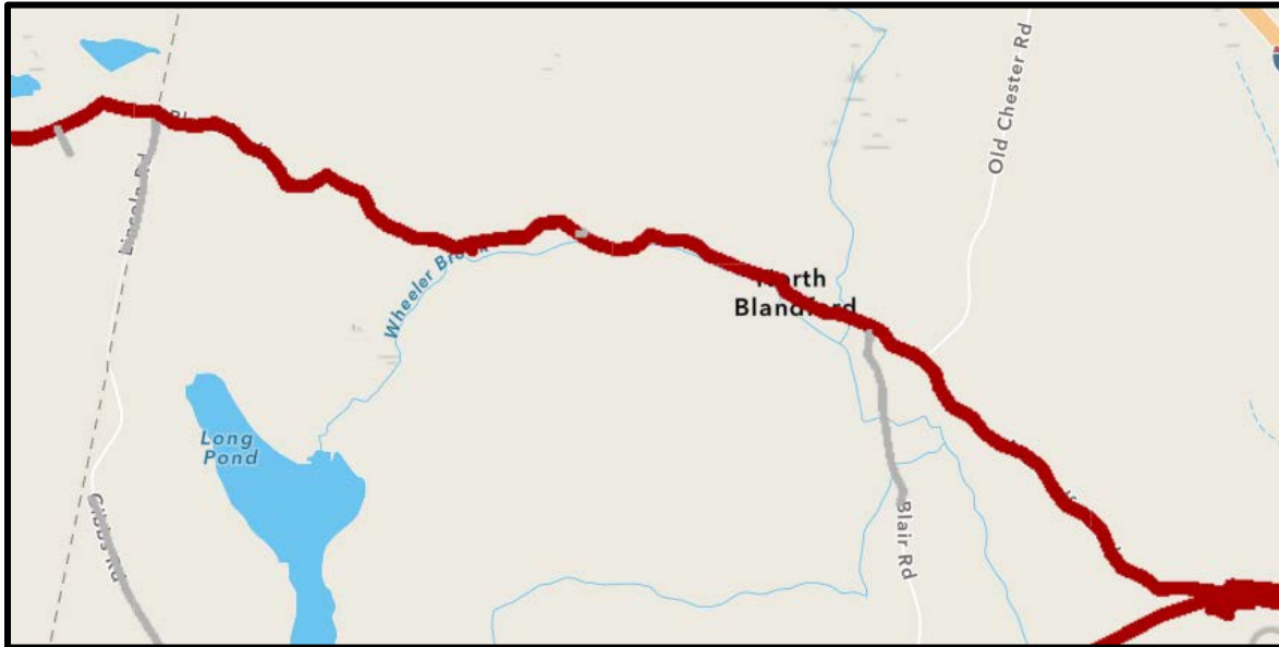
Figure 4 A close-up of the 19J3 feeder circuit, serving North Blandford Road with three-phase power (red line), and Blair and Lincoln Roads with single-phase power (gray lines). Source: Distributed Generation Hosting Capacity Map, Eversource 2020
